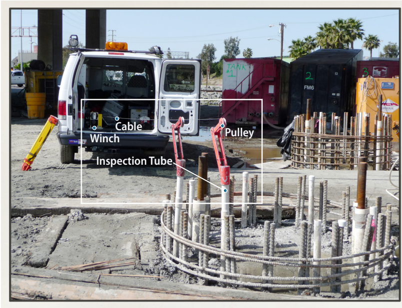
Figure 1 Example of Gamma Gamma Logging at a Construction Site
